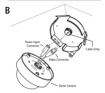
Install the dome camera on the corner mount by first arranging the cables.
